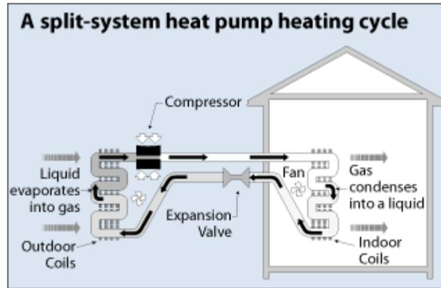
In heating mode, an air-source heat pump evaporates a refrigerant in the outdoor coil; as the liquid evaporates it pulls heat from the outside air. After the gas is compressed, it passes into the indoor coil and condenses, releasing heat to the inside of the house. The pressure changes caused by the compressor and the expansion valve allow the gas to evaporate at a low temperature outside and condense at a higher temperature indoors.
