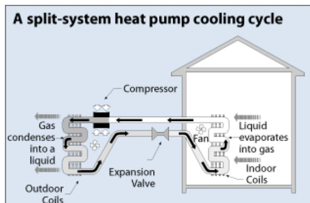
In cooling mode, an air-source heat pump evaporates a refrigerant in the indoor coil; as the liquid evaporates it pulls heat from the air in the house. After the gas is compressed, it passes into the outdoor coil and condenses, releasing heat to the outside air. The pressure changes caused by the compressor and the expansion valve allow the gas to condense at a high temperature outside and evaporate at a lower temperature indoors.
