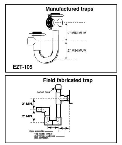
Recommended trap configurations. Illustration from Trane installation manual.
