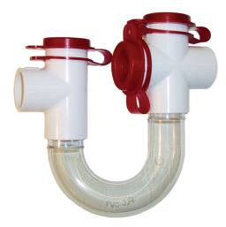
Photo: Recommended by some equipment makers, the translucent EZ Trap® Kit includes a tee and a cross with removable caps and ise packaged with a flexible brush for cleaning. Photo Gerry Spanger, Airtec Products Corporation & Marketair, Inc.
